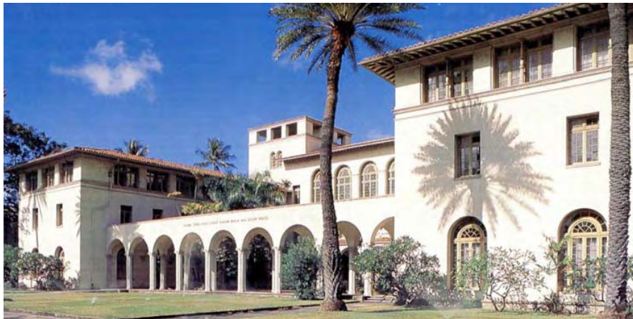
Figure 5.23 - Building Massing Broken Up into Smaller Components
